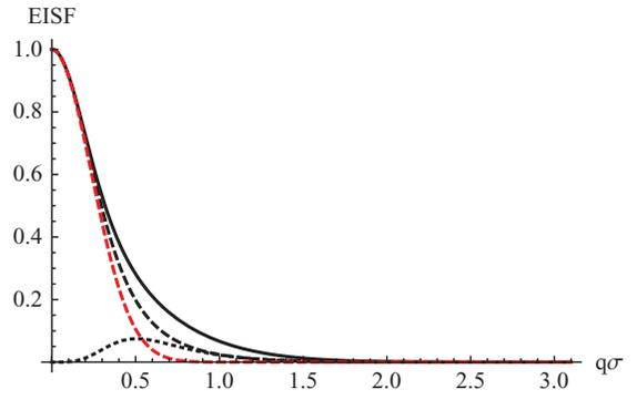
FIG. 2. Model EISF according to (50) for  $\epsilon = 4$  (solid black line), the isotropic term  $\text{EISF}_0(q)$  (black dashed line), and the multipole term  $\text{EISF}_2(q)$  (black dotted line). The red dashed corresponds again to the Gaussian approximation.
