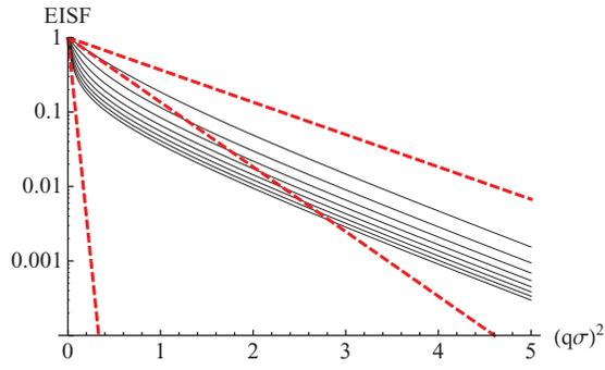
FIG. 1. The solid black lines display  $\overline{\text{EISF}(\mathbf{q})}$  corresponding to model (50) in a log-square plot, where  $\epsilon = 1, 2, \dots, 8$  (from top to bottom). The red dashed lines correspond to the isotropic Gaussian approximation (44) for  $\epsilon = 0, 1, 8$ , respectively.
