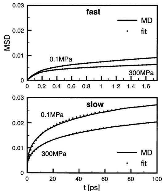
FIG. 2. Average atomic mean square displacement of lysozyme in solution obtained from MD simulation at  $p=0.1$  and at 300 MPa (solid lines). The broken lines correspond to a fit of the model according to expression (3). The panel named “fast” refers to the short trajectory (20 ps,  $\Delta t=0.005$  ps) and the one named “slow” to the long trajectory (1 ns,  $\Delta t=0.040$  ps) (Ref. 16) (see Tables I and II for the resulting parameters).
