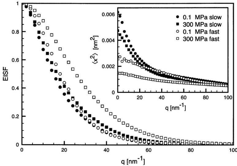
FIG. 1. Simulated EISF of lysozyme for  $p=0.1$  and 300 MPa obtained from the short trajectory (20 ps,  $\Delta t=0.005$  ps  $\rightarrow$  fast) and from the long trajectory (1 ns,  $\Delta t=0.040$  ps  $\rightarrow$  slow) (Ref. 16). The inset shows the position fluctuations derived from expression (10).
