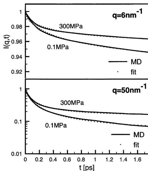
FIG. 3. Simulated incoherent intermediate scattering function (solid lines) obtained from the short trajectory (20 ps,  $\Delta t=0.005$  ps) and fit of expression (6) (broken lines) for  $p=0.1$  and 300 MPa at  $q=6$  nm $^{-1}$  (upper part) and 50 nm $^{-1}$  (lower part). The parameters are given in Table I.
