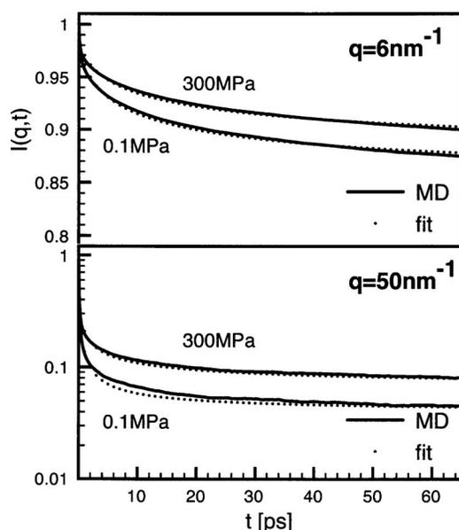
FIG. 4. Simulated incoherent intermediate scattering function (solid lines) obtained from the long trajectory (1 ns,  $\Delta t=0.040$  ps) and fit of expression (6) (broken lines) for  $p=0.1$  and 300 MPa at  $q=6$  nm $^{-1}$  (upper part) and 50 nm $^{-1}$  (lower part). The parameters are given in Table II.
